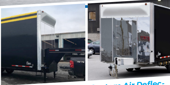
Stainless Steel Skin, Custom Air Deflectors, Man Doors, Extra LEDs
